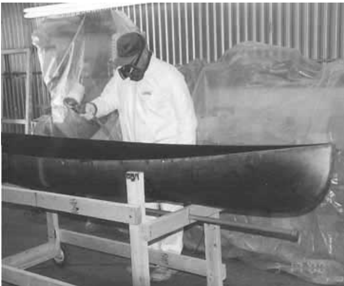
Spraying The Gelcoat
